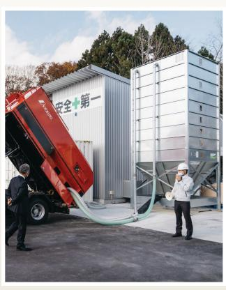
The 60 degree hopper base ensures that the silo drains completely and eliminates the need for periodic cleaning of dust while the look of the square silo fits well with the containerised CHP boilers provided.
