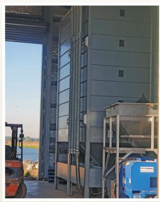
These rectangular silos had two outlets each which were raised approximately 1m off the ground with custom manufactured connections to allow for a conveying auger to take the fish feed from the silos and transfer them into the feeding area of the farm enclosures.
