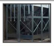
A 60 Degree Hopper Allows for smoother flow of pellets
